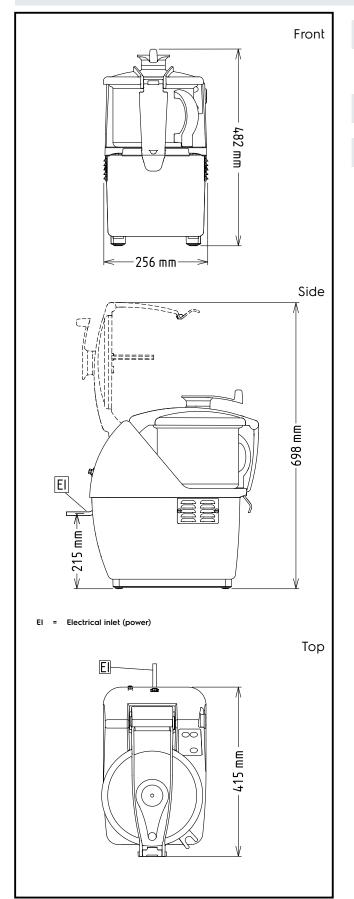
Electric Supply voltage: 602323 (K45VVIJ) 100 V/1N ph/50/60 Hz **Total Watts:** 1 kW Capacity: Capacity: 4.5 litres **Key Information:**
